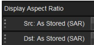
*Display Aspect Ratio* sets the scaling used when *Auto Zoom* is set to **AR**. We can set both *Src* (input) and *Dst* (output).
